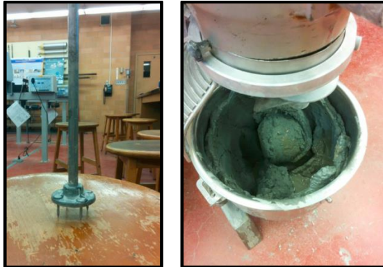
Figure 1. From left to right: compaction rod, Hobart mixing unit homogenizing cement treated clay
