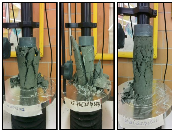
Figure 2. From left to right: conical failure, shear failure, and crushing failure
